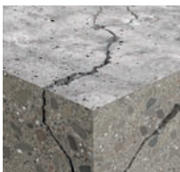
Cracked concrete C20/C25 to C50/C60
